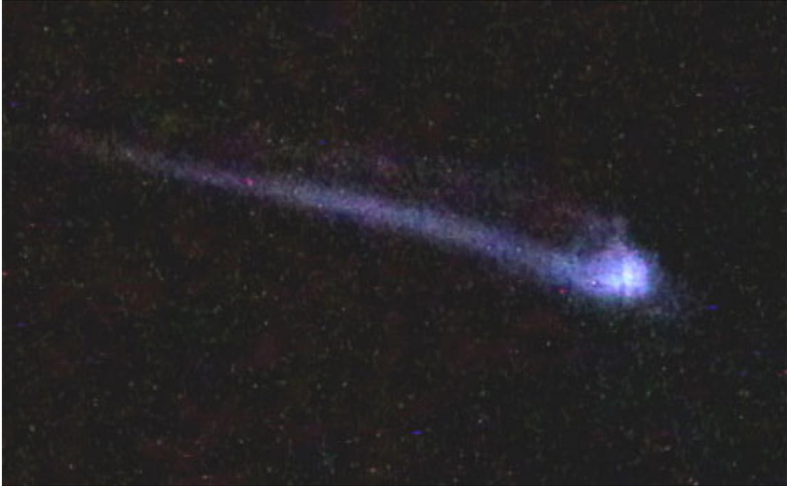
*Figure 15: Single Bubble Sonoluminescence at the bottom node of the cell.*
