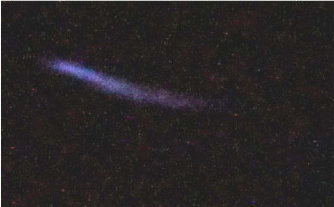
Figure 13 shows the bubbles travelling from the filament to the bottom node of the cell. At this point only a faint glow was visible to the unaided eye, this glow is more visible due to the long exposure used here.
